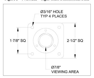
Figure 4 – Full Scale 1" Promate™ Sight Glass Mounting Template NOTE: Make sure this template is printed at 100%.
