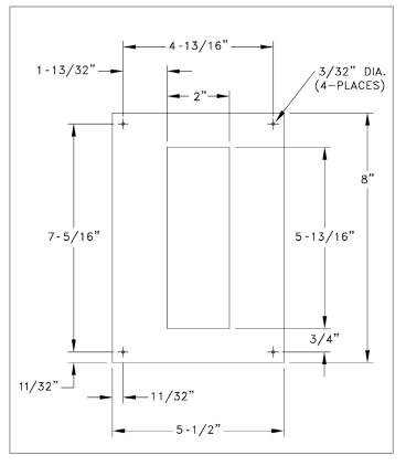
Figure 7 – AD Mounting Template - Full Scale (1-Lamp) NOTE: Make sure this template is printed at 100%.
