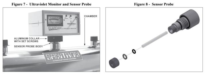
If after cleaning the quartz sleeve, there is no significant improvement in the ultraviolet intensity, as shown on the intensity meter, it may be necessary to clean the Ultraviolet Monitor's sensor probe. The sensor probe body mounts in a fitting, located in the center of the disinfection chamber, and protrudes into the chamber.
