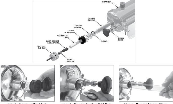
Figure 5 - Quartz Sleeve Installation or Replacement (SANITRON® MODEL S37C Shown)
