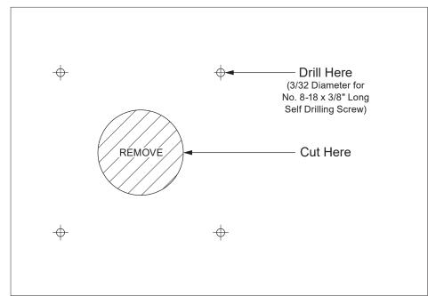
Figure 5 – Sight Glass Mounting Template – Full Scale <u>NOTE</u>: Make sure this template is printed at 100%.
