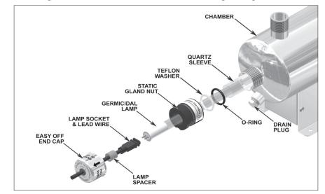
Figure 5 – Quartz Sleeve Installation, Cleaning, or Replacement
