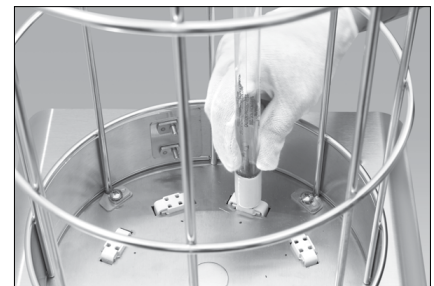
Step 4 – Insert Lamp into Socket
