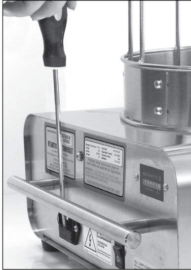
Step 1 – Insert Screwdriver & Bring Tray Forward
