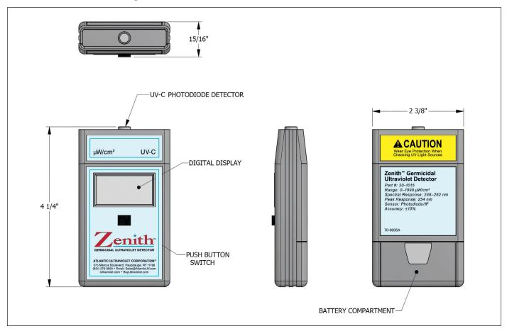
Shown in **Figure 1**, the **Zenith™** Germicidal Ultraviolet Detector consists of the following:
