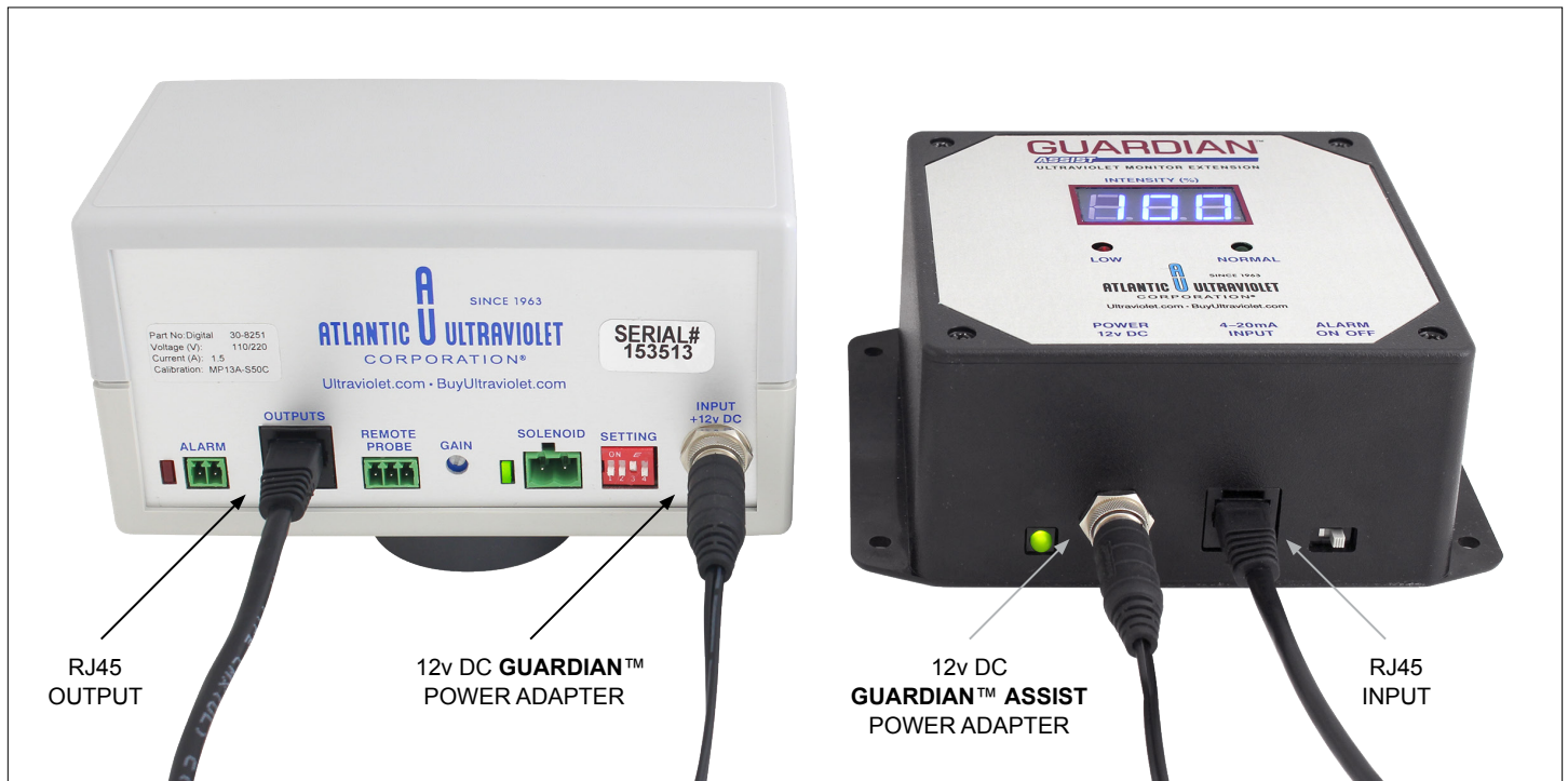
Figure 4 – Connecting GUARDIAN™ ASSIST to the Digital GUARDIAN™ Ultraviolet Monitor
