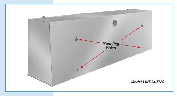
**Figure 1 –** Shows the back side of **Hygeaire® Model LIND24-EVO**; note the four mounting holes in the back of the fixture. The fixture is to be mounted on a plumb and vertical surface, at a minimum height of 7 feet from the bottom of the fixture to the floor, in a location that must be able to safely support 16 pounds.
