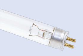
**STER-L-RAY**® **Germicidal UV Lamps** are shortwave, low pressure tubes that produce ultraviolet wavelengths lethal to microorganisms. Approximately 95% of the ultraviolet energy emitted from **STER-L-RAY**® Germicidal Ultraviolet Lamps is at 254 nanometers, the region of germicidal effectiveness most destructive to bacteria, mold and virus.
