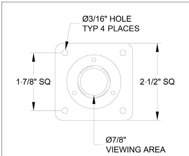
Figure 4 – Full Scale 1" Promate™ Sight Glass Mounting Template
