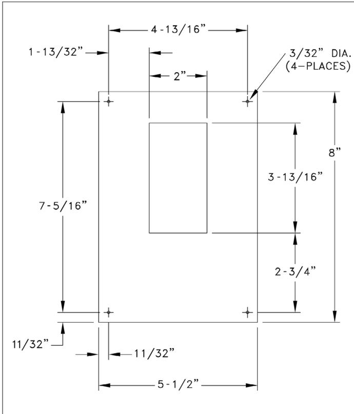
Figure 6 – AD Mounting Template
