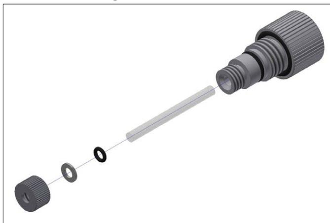
If after cleaning the quartz sleeve, there is no significant improvement in the ultraviolet intensity, as shown on the intensity meter, it may be necessary to clean the Ultraviolet Monitor's sensor probe. The sensor probe body mounts in a fitting, located in the center of the disinfection chamber, and protrudes into the chamber.
