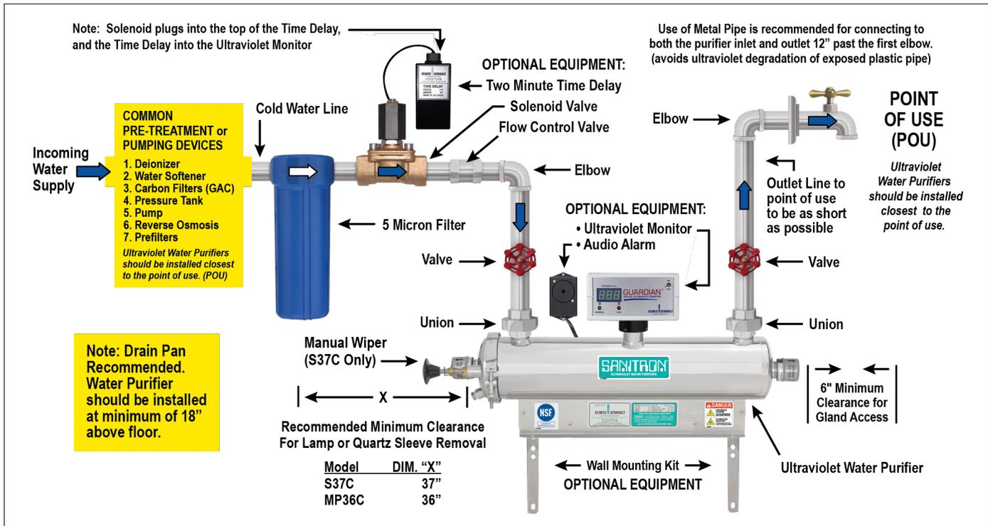
3. The water purifier should be mounted horizontally on a flat dry surface. Secure the water purifier using the mounting holes in the ballast housing or with the optional wall mounting kit. The purifier should not be solely supported by its plumbing connections.
