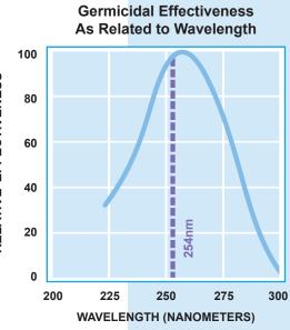
Approximately 95% of the ultraviolet energy emitted from **STER-L-RAY**<sup>®</sup> germicidal lamps is at 254 nanometers, the region of germicidal effectiveness most destructive to bacteria, mold, and virus.
