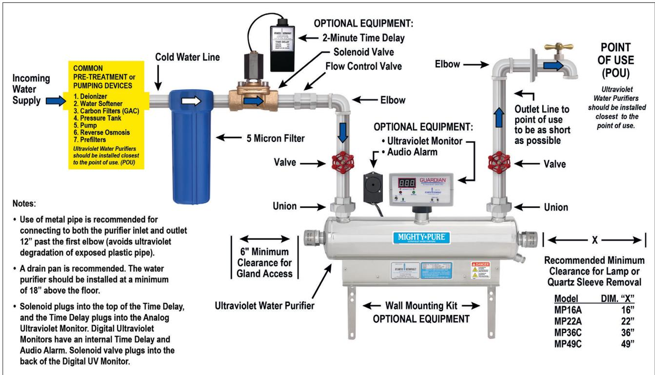
3. The water purifier should be mounted horizontally on a flat dry surface. Secure the water purifier using the mounting holes in the ballast housing or with the optional wall mounting kit. The purifier should not be solely supported by its plumbing connections.
