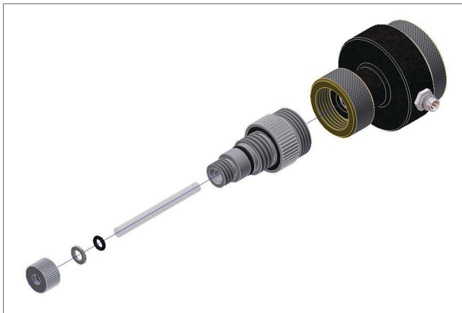
Figure 15 – Removing Quartz Rod from Remote Probe
