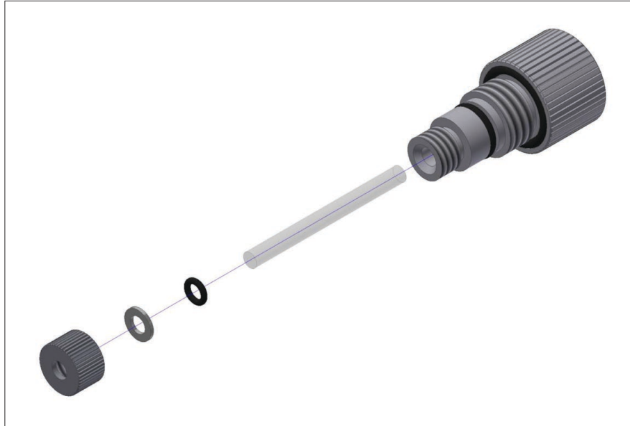
Figure 15 – Removing Quartz Rod from Remote Probe
