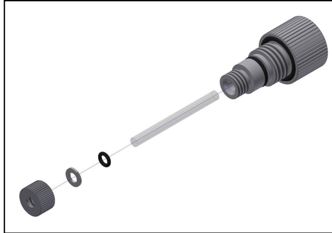
Figure 9 – Removing Quartz Rod from Standard Probe
