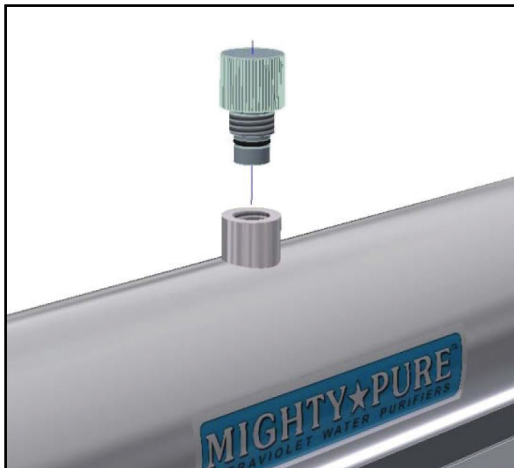
Figure 4 – Removal of Sight Port Plug
