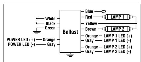
\*For 3-wire output application, cap Blue lead and insulate to 600v.
