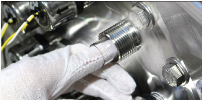
Step 8: With One Person Supporting Quartz Sleeve with a Finger, Have Other Person Carefully Remove Quartz Sleeve
