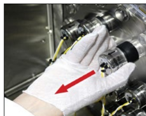
Step 3: Remove Lamp 4" / Remove Lamp Socket
