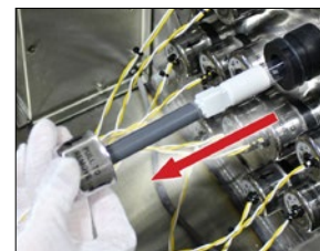
Step 3: Remove Lamp 4" / Remove Lamp Socket
