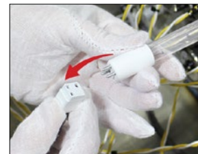
Step 4: Carefully Remove Lamp Completely
