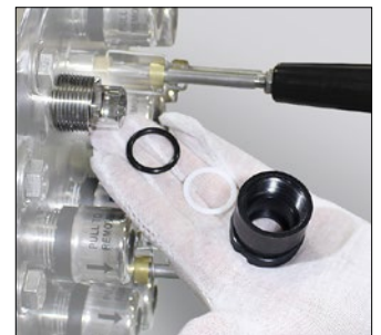
Step 8: With One Person Supporting Quartz Sleeve with a Finger, Have Other Person Carefully Remove Quartz Sleeve
