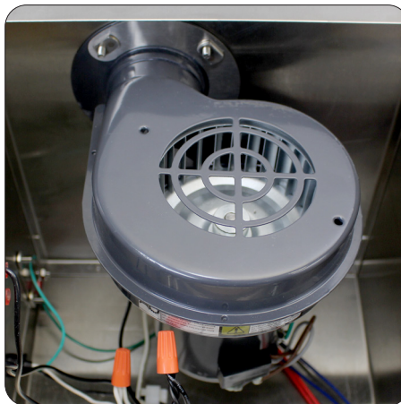
Figure 8 – Completed Blower Assembly
